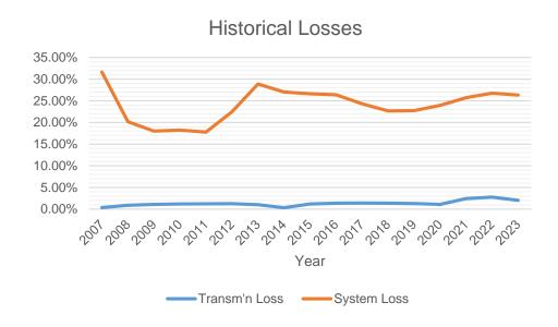
Historically, Transmission Loss ranged from 0.30% to 2.76% while System Loss ranged from 17.76% to 31.64%. Transmission Loss peaked at 2.76% on year 2022 while System Loss peaked at 31.64% on year 2007.
