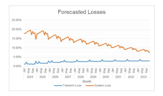
Transmission Loss is expected to range from 1.08% to 3.70% while System Loss is expected to range from 7.35% to 19.55% over time.
